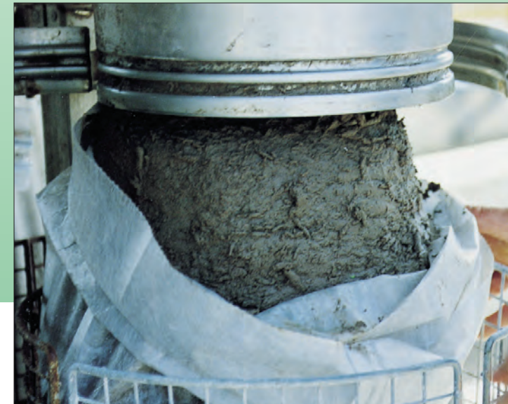
Sludge dewatered after 24 h
